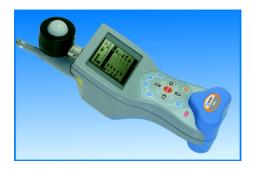
Measurement functions for air temperature, air velocity, relative humidity, illluminance and luminance are all found within one device.
